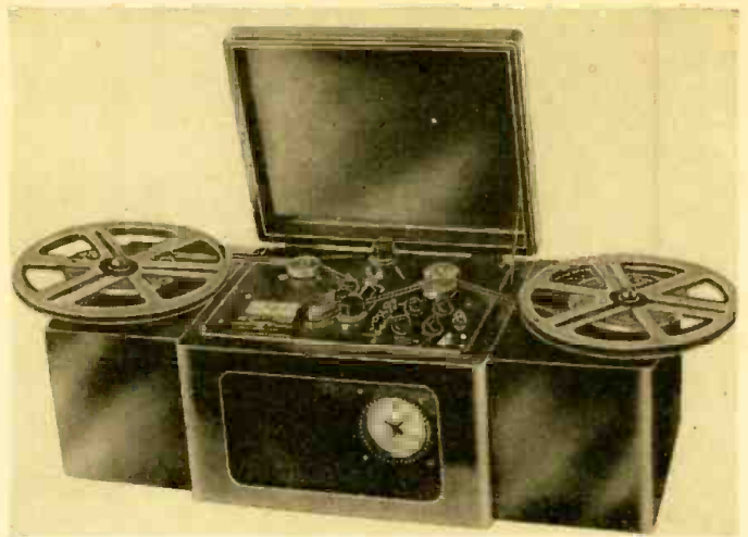
9-tube amplifier is housed in this long-playing recorder-reproducer.
